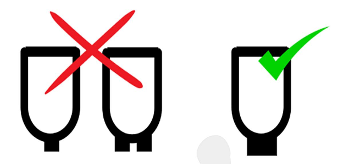
Use the correct stand which must be central and support the whole base
