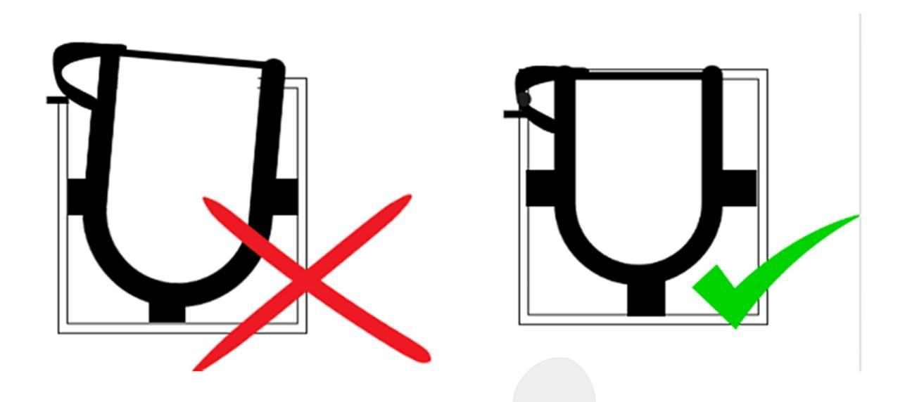
Use correctly positioned grip bricks in tilting furnaces, leaving gaps for expansion. Do not hang it on spout
