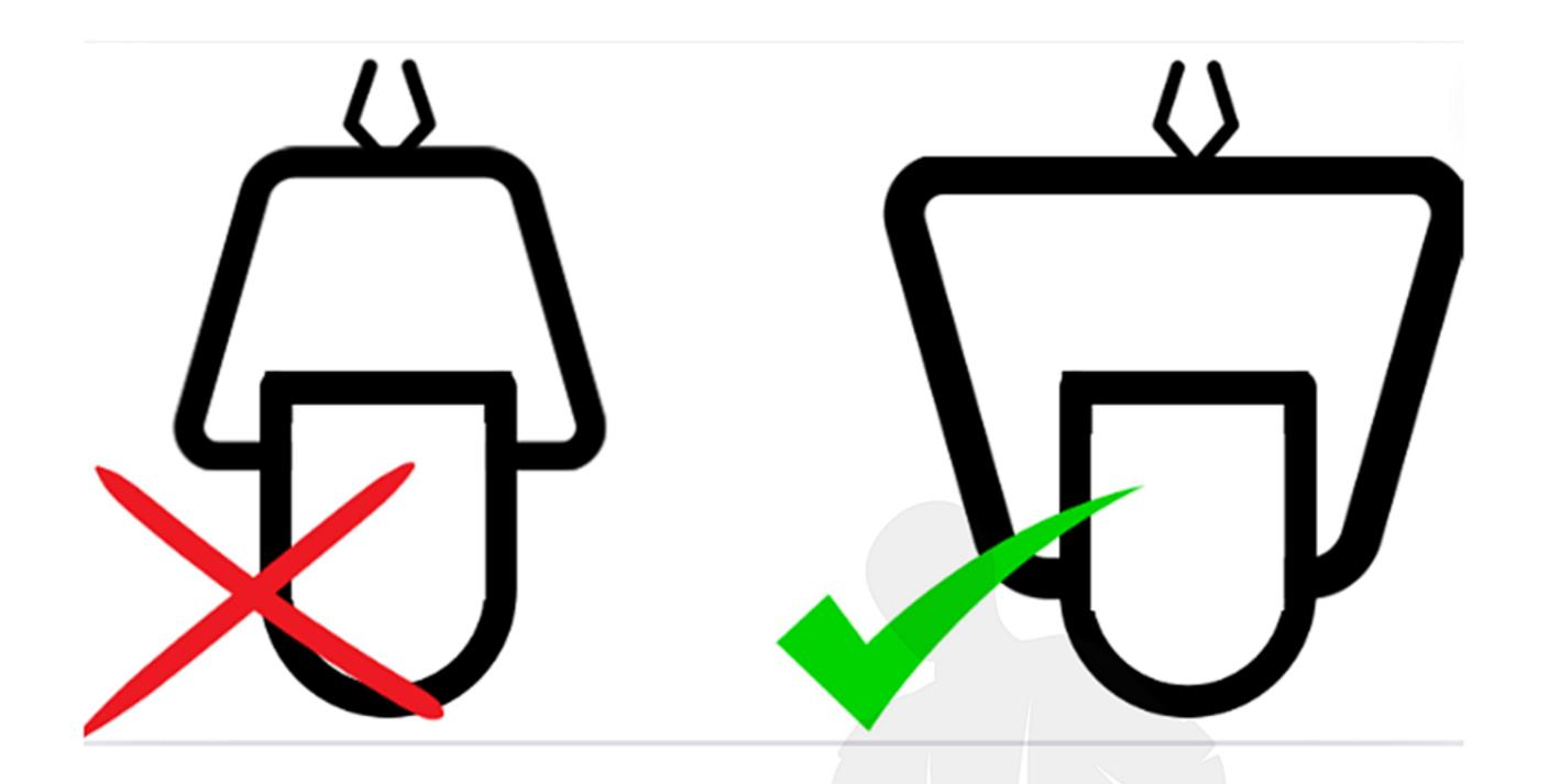
Lift-out tongs should hold on its lower third and fit evenly on both sides
