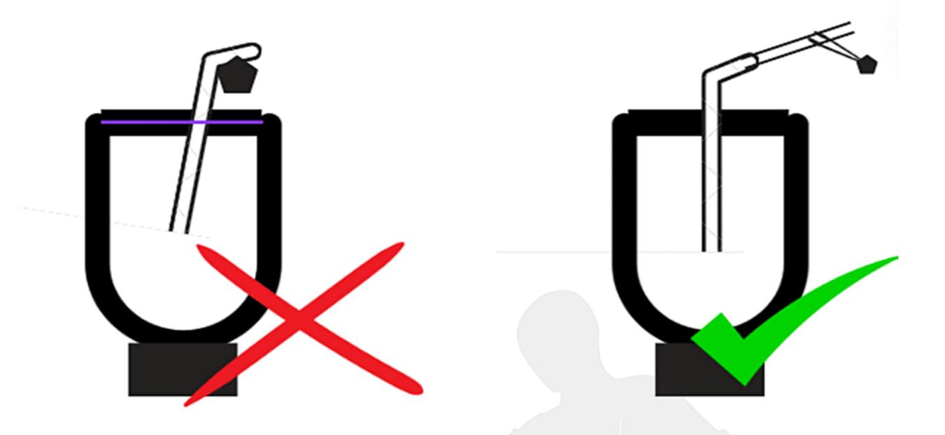
Ingots should be loaded carefully using tongs
